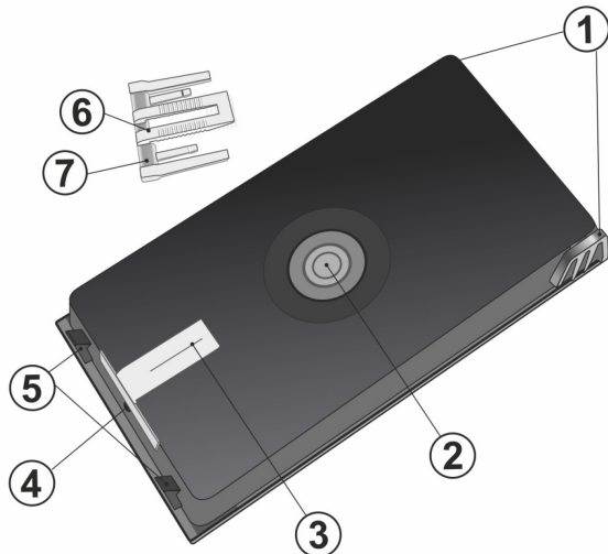
Fig. 1: Panic button in its mounting platform: 1. Hinges, 2. Button A, 3. Switch B, 4. Backplate fixing screw, 5. Mounting platform latches, 6. Replaceable banknote or document clip, 7. LED light guide.
