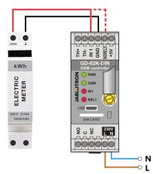
Figure 6: Electricity consumption measurement mode.
