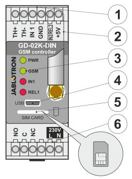
Figure 1: 1 – Low voltage terminals; 2 – GSM antenna; 3 – LED indicators; 4 – MicroUSB connector for connection to PC; 5 – SIM card slot; 6 – Power output relay terminals and 230 V mains terminals.
