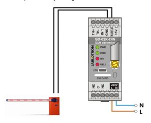
Figure. 2: GD-02K-DIN as a gate controller.
